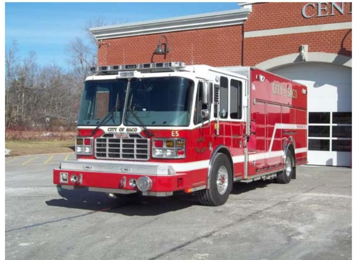
Engine 5 was designed to meet the increasing responsibilities assigned to the fire department and it is better suited for our large volume of calls that are not fire suppression related. The focus is shifting from carrying large amounts of hose to increased compartmentation for effective and efficient operations at medical calls and specialized rescues as well as its' ability to operate as a fully functional pumper at a fire scene; hence the term Multi-Vocational Pumper
