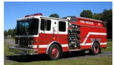
Side mount pumper with a seating capacity of 5, a 1250 GPM (Gallon Per Minute) pump 1000 gallon tank, Class B 55 Gallon foam tank and 8 SCBA Units (Self Contained Breathing Apparatus)
