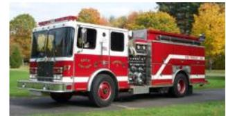
Side mount pumper with a seating capacity of 5, a 1250 GPM (Gallon Per Minute) pump 1000 gallon tank, Class B 55 Gallon foam tank and 8 SCBA Units and carries our Holmatro Extrication System & vehicle stabilization equipment systems. Engine 7 is primary for accidents & Hazmat responses
