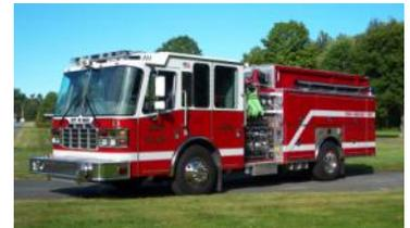
Side mount pumper with a seating capacity of 6, a 1500 GPM (Gallon Per Minute) pump 1000 gallon tank, Class A and Class B foam tanks and 11 SCBA Units (Self Contained Breathing Apparatus)
